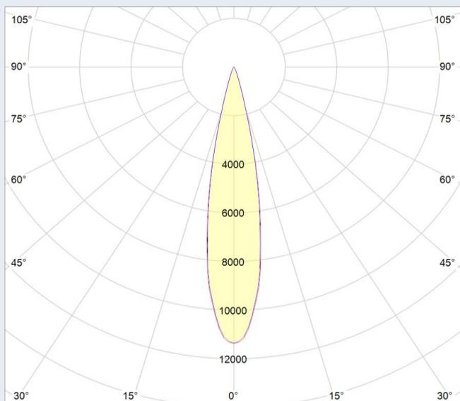
Beam angle (FWHM) measured with Luminus
